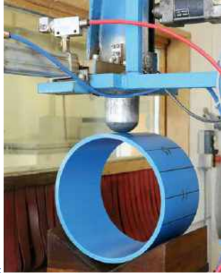
Ball drop test (step method) at -10°C
