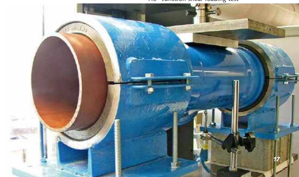
HS®-Junction shear loading test
